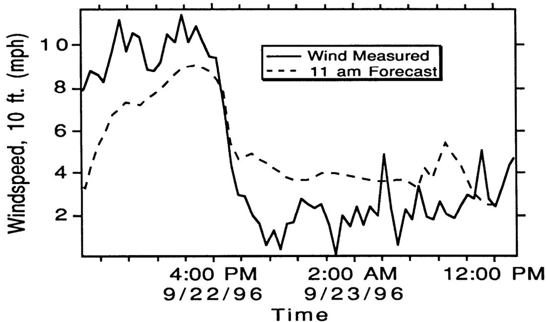
Figure 3. TiSDat automated forecast of the wind at 10 feet above the crop surface.
