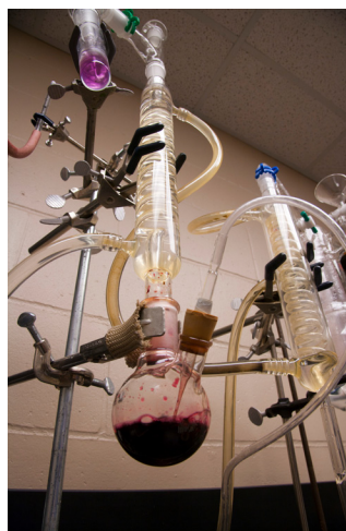
This photo from the Enology Lab at the University of Minnesota shows the aeration/oxidation method of checking free sulfur in wine. Red wine is in the "bulb" at the bottom, air is bubbled through, and it reacts with hydrogen peroxide in the top with a color indicator. The indicator changes from olive green to purple as the SO 2 concentration increases.
