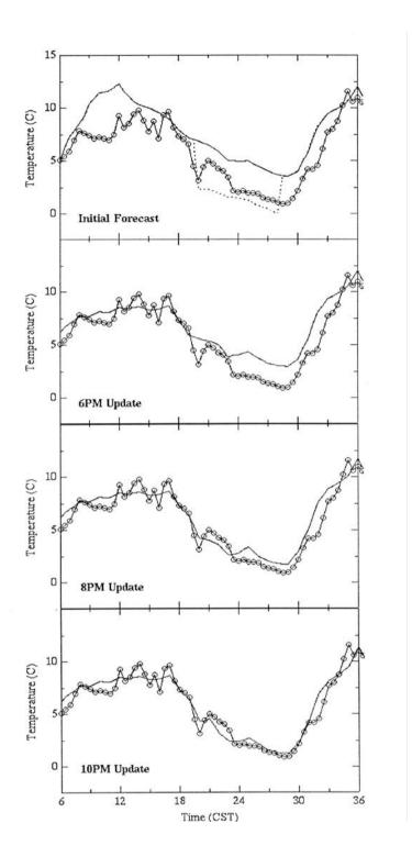
Figure 1: Effect of updates on minimum temperature forecast accuracy. Circles indicate measurements of bog temperature made with our automated weather station at Cranmoor; solid lines indicate the updated forecast at the time specified. The dotted line in the first frame shows a forecast assuming the skies will be clear overnight.
